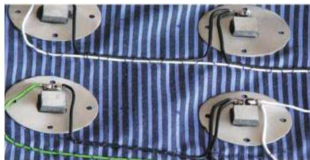
Fig.5. Shows the additional polyester textile used to assemble four of sixteen thermopiles. They were sewed together and were hidden inside the polyester underwear.
