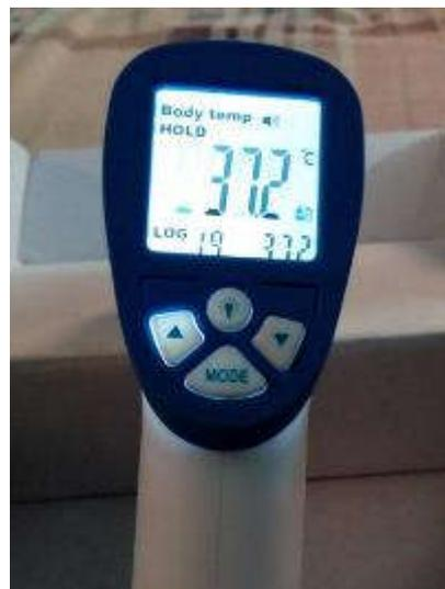
*Fig 4: temperature display on prototyped NCIT*
