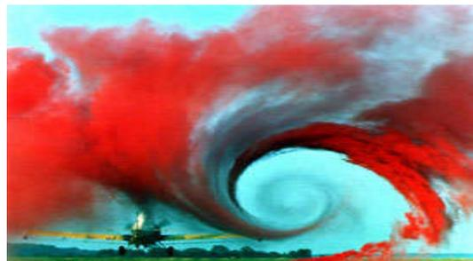
Figure 2: The Structure of a Roll-up Vortex Wake behind a Crop Duster, [17]
