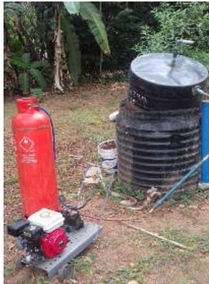
*Fig 1: Set up for harvesting of raw biogas*
