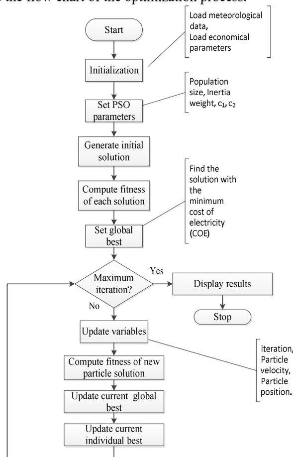
Figure 5: Flowchart of the optimization process using PSO
