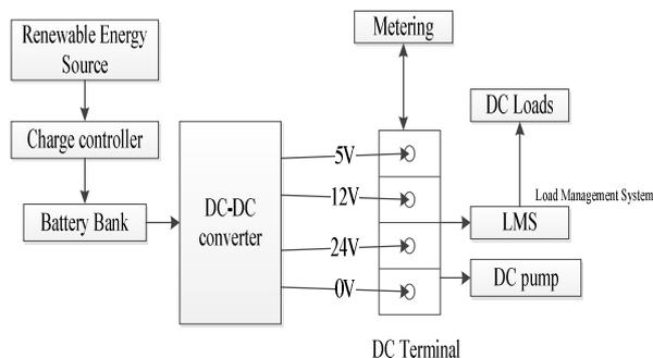
Figure 4: System block diagram showing their interconnectivity
