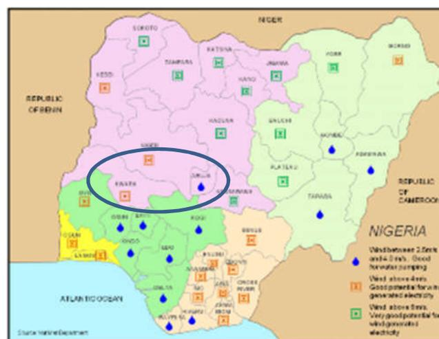
Figure 1: Wind energy potential of different location of Nigeria [11].
