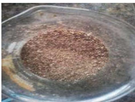
*Fig. 2. Grinded orange peels waste*
