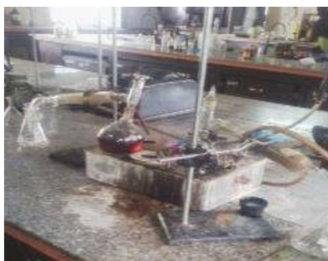
*Fig. 7. 2<sup>nd</sup> Distillation process of ethanol using water bath*
