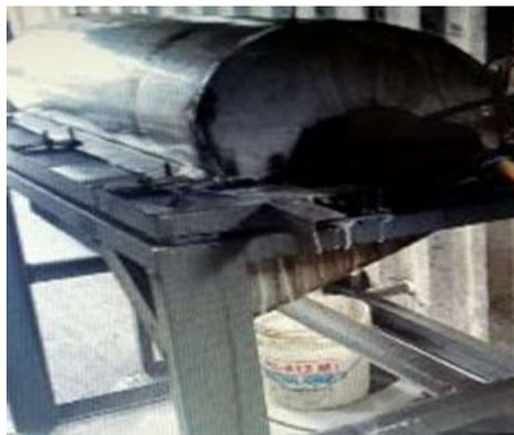
Fig.11. A snapshot of the decanter during operation, the whitish water is the clearer centrate
