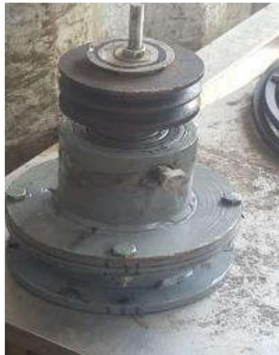
*Fig.9. Epicyclic gear box, front bearing house and differential drive pulley*
