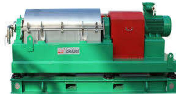
Fig. 3. A view of commercial decanter centrifuge [2]
