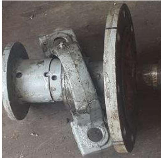
*Fig.8. Front flange and bearing, the smaller flange connect the epicyclic gearbox*
