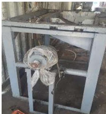
*Fig.10. Frame, the differential drive motor, upper frame mounted on the main frame via 4 rubber damper.*
