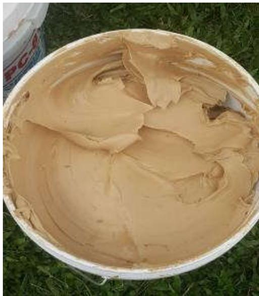
*Fig.15. Sample of cake collected from the decanter centrifuge.*
