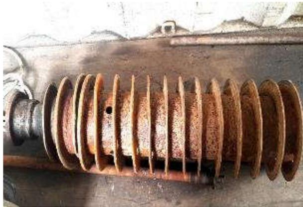
*Fig. 7: A view of the scroll outside the bowl, the feed tube could be seen in the picture next to the scroll*
